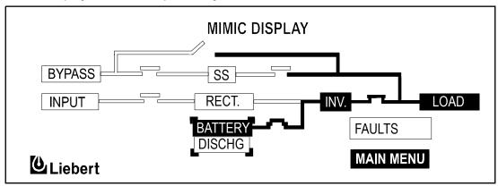
In this example, we see that a utility failure has shut down both the normal and bypass power sources. The battery is connected and supplying power to the load.
